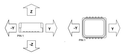
Figure 2. Accelerometer measuring directions
