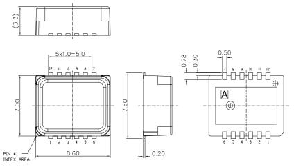
Figure 3. Housing dimensions
